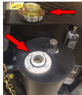
hydraulic oil tank (15)
